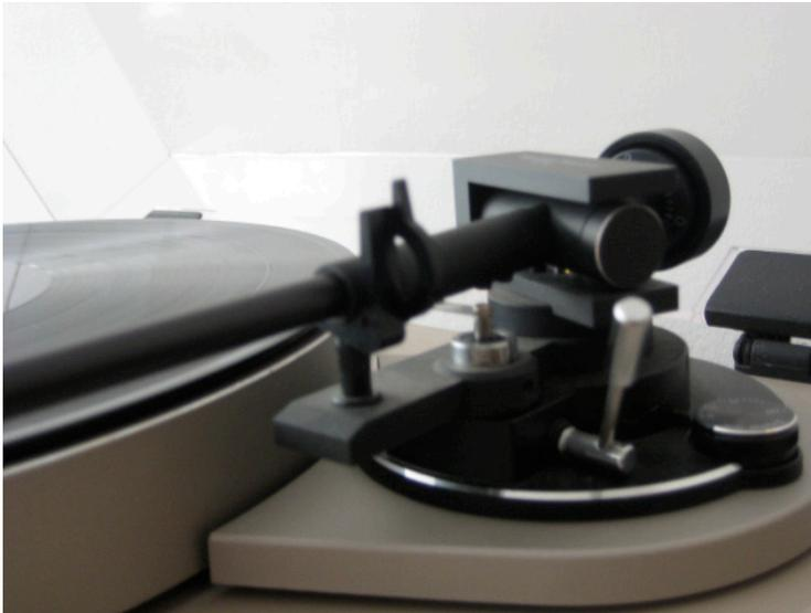
The movement of the handle that controls the tonearm on this turntable is constrained to up and down movement. There is a physical constraint that limits the range of options available for operating this object. The movement of the handle that corresponds to the movement of the tonearm is also an example of clear natural mapping. Newer turntable models often employ automatic control which, apart from being bad for records, is not as intuitive.
