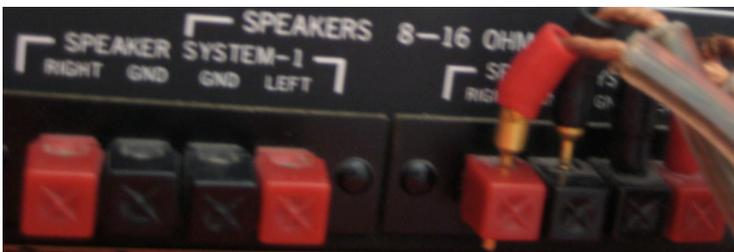
The front plate of this receiver has two push buttons which relate to two sets of speakers. The left one turns the first set on while the right one turns the second set on. On the back panel though the first set of speakers is on the right side. Does this layout reflect natural mapping?
