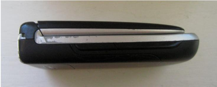
The volume control on this cell phone is placed on the side and its color blends with the casing. It's practically invisible and very easily unintentionally activated. It is actually just one button. If pressed closer to the top of the phone volume goes up and vice versa. In this respect it does reflect natural mapping, but it is almost impossible to know which side of the button is going to be pressed.
